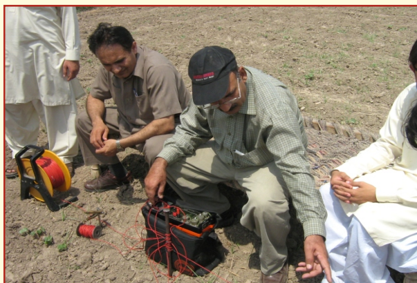
Assessment of aquifer thickness by Resistivity meter
